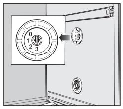
Use a coin or screwdriver to adjust the water hardness selector. There is a click as each setting is reached.
